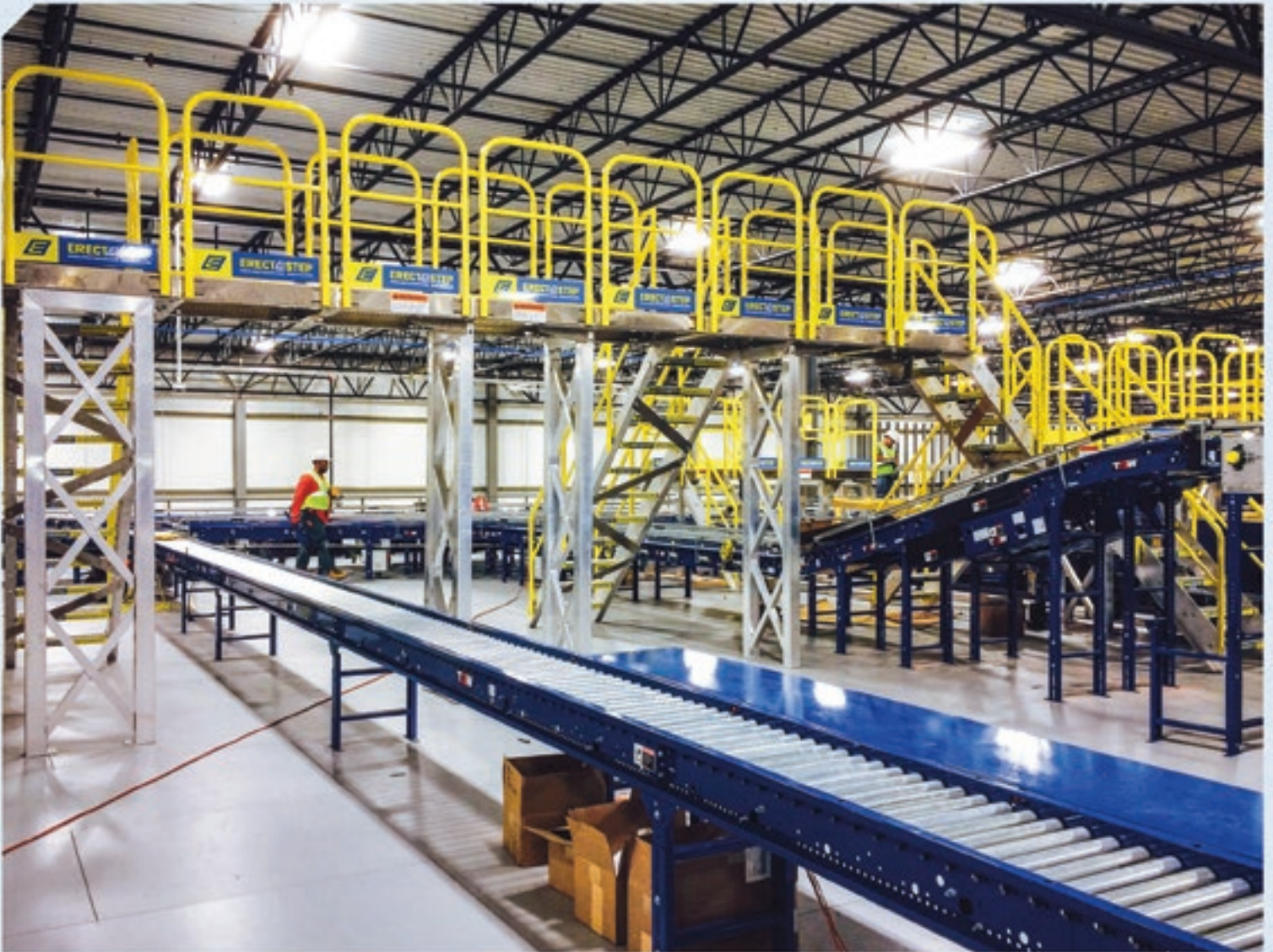
Brand new flagship distribution center crosses over 5000 ft (1524 m) of conveyer with all standard components.
