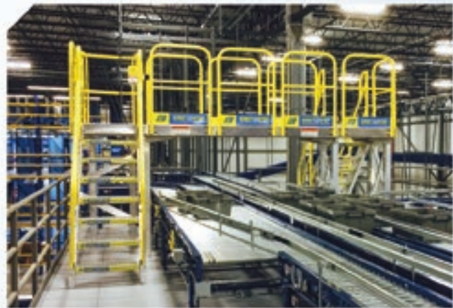
Span 9' (2743 mm) of conveyor with no intermediate support.
