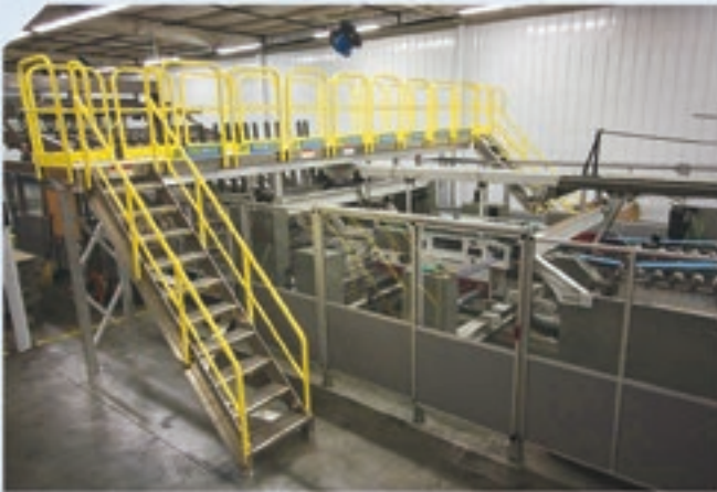
Cross over with 26' (7925 mm) span.
